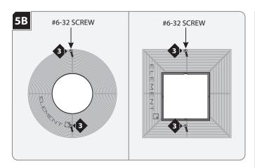
Secure the plaster ring in place with the two provided flat head #6-32 screws. Make sure that the screws penetrate through the drywall into the housing screw holes.
